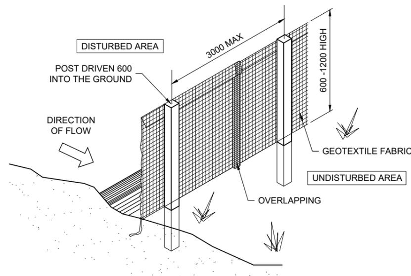
**SEDIMENT AND EROSION FENCE DETAIL**
