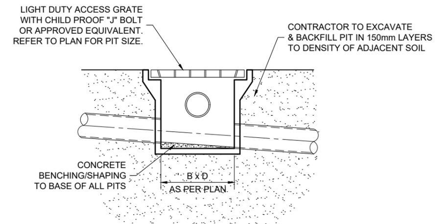
**TYPICAL SURFACE INLET PIT DETAIL**
